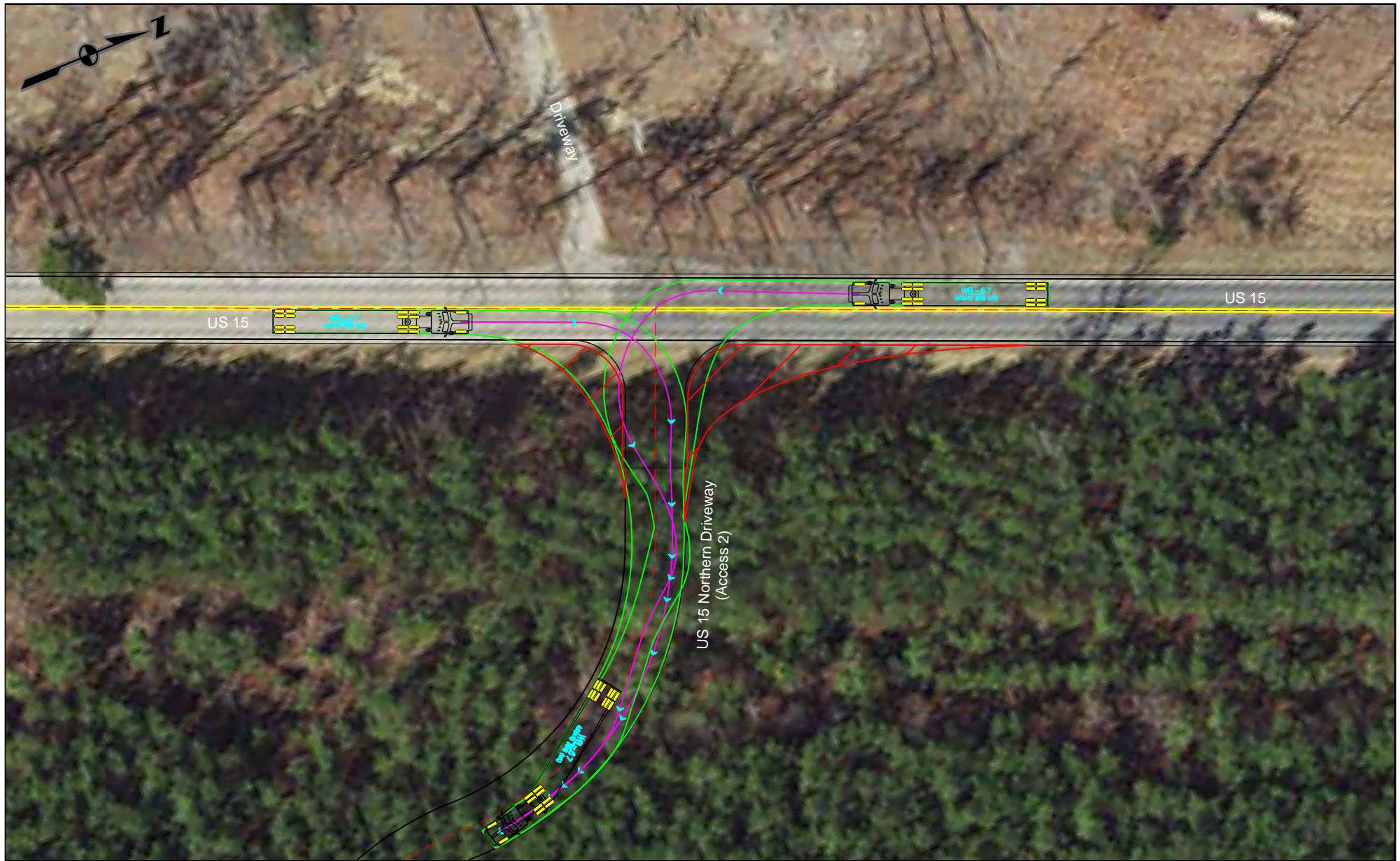
FIGURE 10A AUTOTURN WB-67 SIMULATION US 15 NORTHERN DRIVEWAY (#2) - ENTERING
